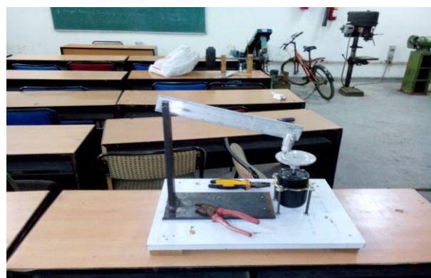
Fig 3: Construction of the wear testing machine
